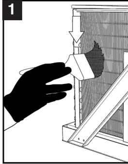
1. Use a long bristled brush in a vertical sweeping motion to remove lint, dust and debris from in between the metal fins of the condenser coil. Do not apply heavy pressure so as not to bend the fins.
