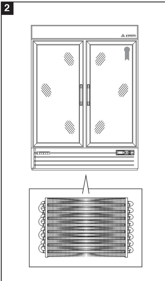
2. The condenser coil is behind the vented grill at the bottom of the unit.
