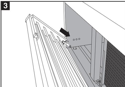
3. Lift the vented grill vertically until the two keyholes on its bottom edge clear the stationary bolts.
