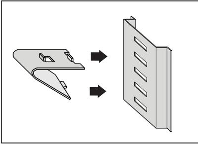
1. Attach the shelf clips onto the pilasters by inserting its top hook into a pilaster notch followed by the bottom hook. Do not use pliers or other crimping tools to modify the shape of the shelf clips. This will result in shelf mounting instability.
