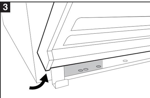
3. Lift the vented grill vertically until the two keyholes on its bottom edge clears the stationary bolts.
