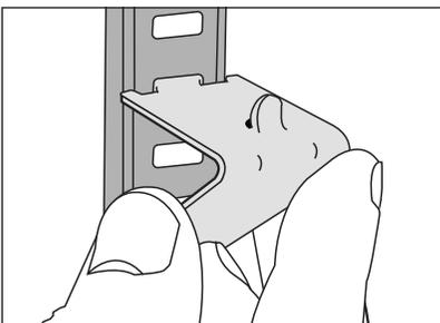
3. When removing a shelf, unmount the shelf from the shelf clips. To detach the shelf clip from the pilaster, tilt up the shelf clip until the bottom hook clears, followed by the top hook.
