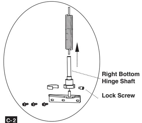
4. Locate the door spring shaft on the top right corner of the door **C-1**. The head of the shaft has 4 screw holes, one of which is occupied by a lock screw that maintains door spring tension **C-2**. Remove the half ring shaft cap to expose the remaining vacant screw holes.
