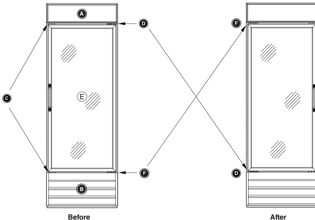
1. The top signboard (A) and front bottom grill (B) must be removed to access the door hinge mounting screws. Detach the top signboard by removing 3 top and 2 bottom screws.
