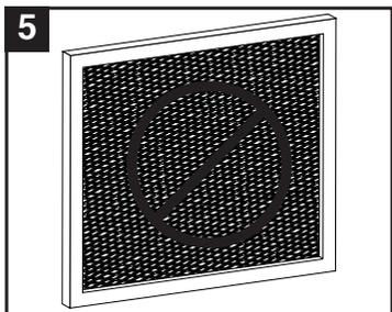
5. Do not attach an aftermarket filter or screen around the condenser coil. This obstructs ventilation which leads to overheating, component failure or the risk of fire.
